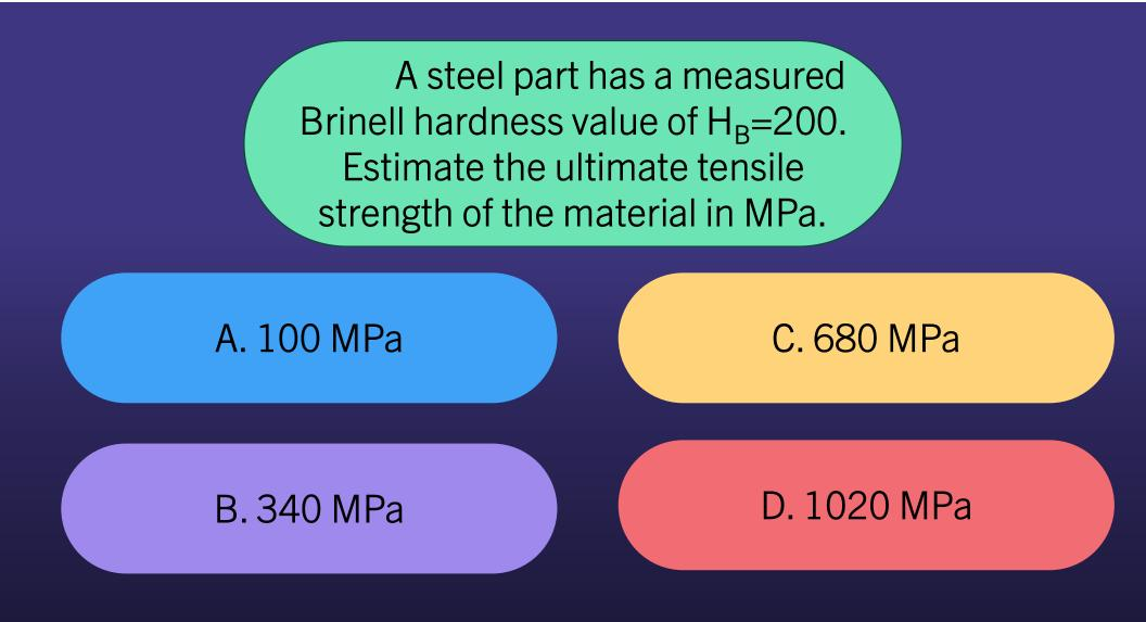
A steel part has a measured Brinell hardness value of  $H_B=200$ . Estimate the ultimate tensile strength of the material in MPa.
